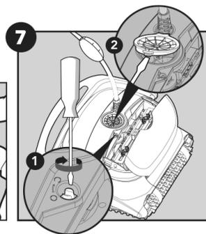
Dismantle the impeller cover and clean around the impeller housing, then reassemble.
